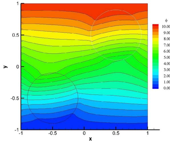
Fig. 4. IFE solution for conducting cylinders with PBC.
