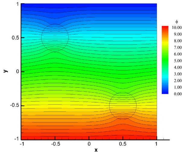
Fig. 6. Symmetric partially penalized IFE solution for conducting cylinders with homogeneous flux jump.
