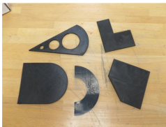
Figure 11 - At Highworth Grammar School for Girls, a set of laminae were made to support the teaching of centres of mass in mechanics instruction.
