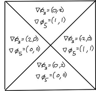
The gradients are constant vectors. In  $e_1$ ,  $\nabla\phi_3 = \langle 0, 2 \rangle$ , in  $e_2$ ,  $\nabla\phi_3 = \langle 2, 0 \rangle$ , in  $e_3$ ,  $\nabla\phi_3 = \langle 0, -2 \rangle$ , in  $e_4$ ,  $\nabla\phi_3 = \langle -2, 0 \rangle$ . Similarly In  $e_1$ ,  $\nabla\phi_5 = \langle 0, 0 \rangle$ , in  $e_2$ ,  $\nabla\phi_5 = \langle 0, 0 \rangle$ , in  $e_3$ ,  $\nabla\phi_5 = \langle 1, 1 \rangle$ , in  $e_4$ ,  $\nabla\phi_5 = \langle 1, 1 \rangle$ .
