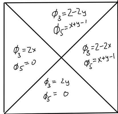
where  $\partial\Omega$  is the boundary of the unit square, and  $\vec{n}$  is the outer unit normal. Because  $\phi_3$  is zero on the boundary, the boundary term just disappears. We are left with the second term.
