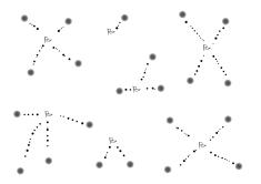
Sensors with limited range are placed through an area. Local receivers are placed to record and package data  $(P_i)$ .
